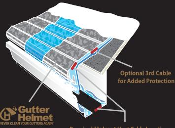
Required Helmet Heat Cable Locations Includes Downspouts
