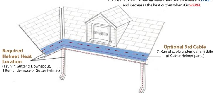
The Helmet Heat System increases heat output when it is COLD...
